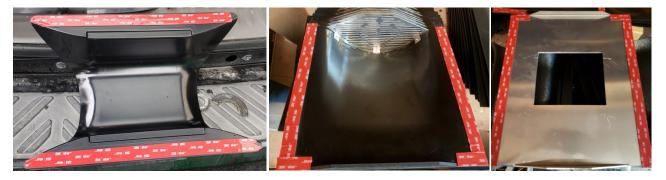
5) Press well to make sure initial contact is made. Cure is secure at 40% (after 20 minutes). The "Exhaust Driver" has two parts, port then cover. Intake has one part. The 3M tape takes about 24 hours to cure completely.
