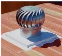
A wind powered 12" rooftop turbine, has a draw rate of about 8 cu ft / min / 1 mph. It will provide about 22 complete air exchanges on a 40 footer with a daily 5 mph wind. The down side is, it's a difficult install on a corrugated roof, it has no bug screen, and has a mechanical failure component. Made of metal, this is another place for condensation to form. Wind driven mechanical devices have both, a low and high wind threshold. It will not exhaust with thermals. Intake required
