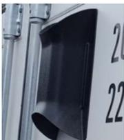
Our wind powered "Wall Exhaust" has a draw rate of about 4 cu.ft / min / 1mph. Provides about 11 air exchanges with a daily 5 mph wind. It would take two vents on a 40' conex to provide sufficient air exchanges for controlling condensation (equivalent of the Turbine). It's an easy install, gains draw rate with turbulence and thermals. Intake required
