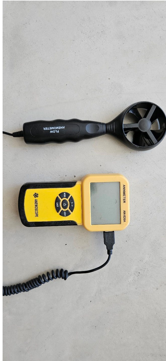
Figure 7: Anemometer air flow device
